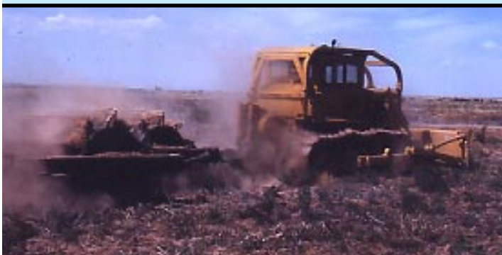
Figure 8. Roller chopping reduces noxious brush and increases forage production through its influence on the water availability.
